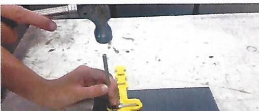
8. Check that the gold rivet has flattened out, securing the key in place.
