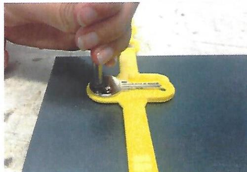
7. Hit the top of the punch several times with a Hammer.
