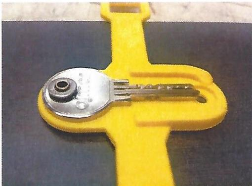
6. Line up the punch so that the flat end of the punch is facing upwards and the other end has slotted inside the top of the rivet.
